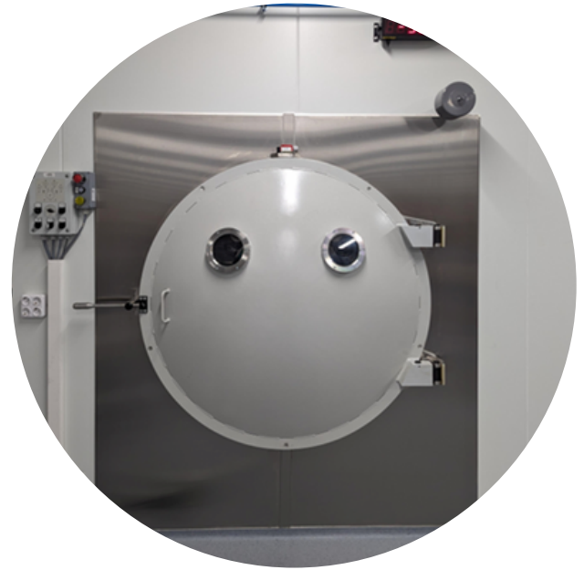
Figure 3: New cutting-edge full-vacuum Li-Metal coater equipment in the ABEE's dry room facility
